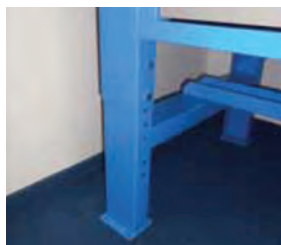
One of the main advantages of the new work benches are the height-adjustable legs.
